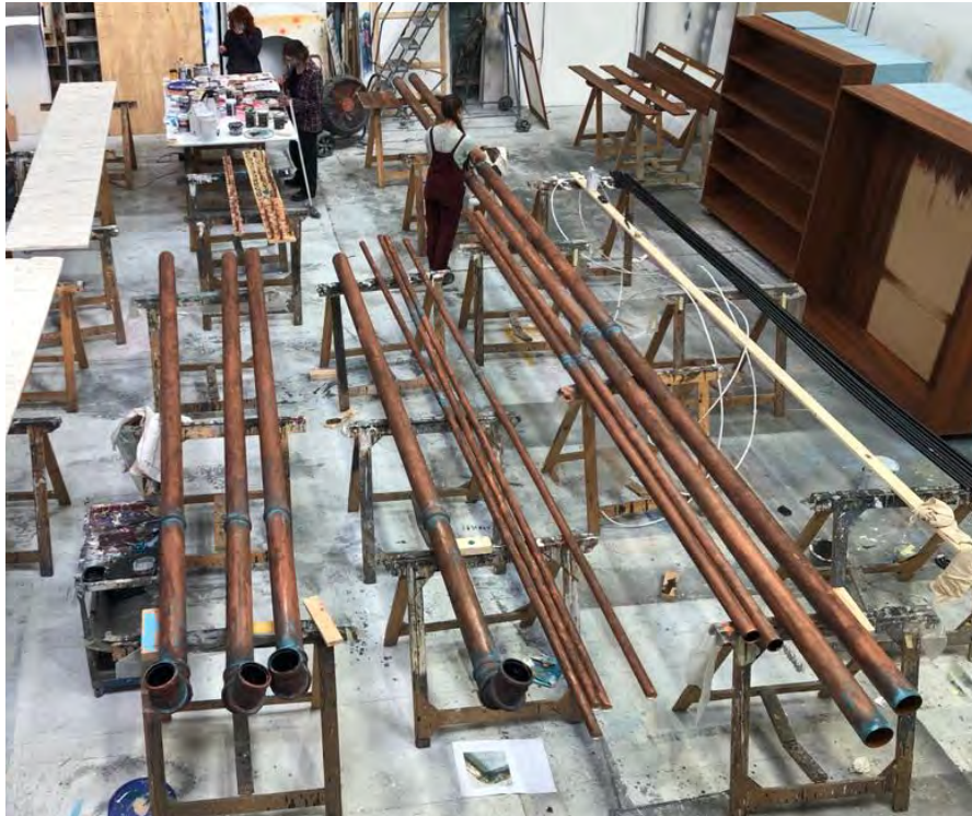
Large copper pipes painted using rollers and metallic powder paint. Vermiculite painted on using natural sponges and brushes
